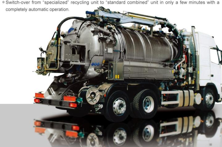
The recycling system allows to recollect and use, after proper filtering, the water of the high pressure
